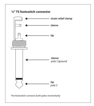
Fig. 4.1:  $\frac{1}{4}$ " TS connector for foot switch
